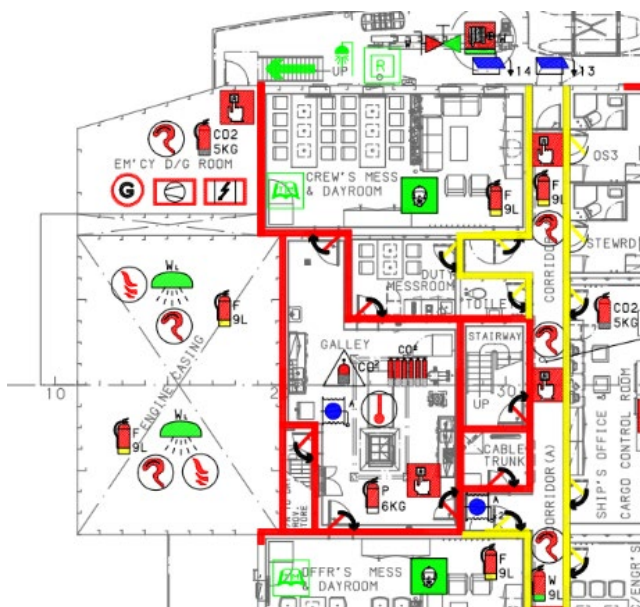
Extract from the main living area of a typical chemical tanker. The detectors and fixed systems for the engine room and galley can be clearly seen.
