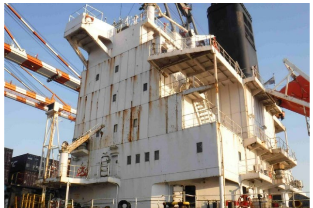
Up to approximately 5% scattered corrosion, mainly at weld seams with subsequent corrosion staining
