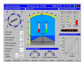
It is difficult to identify these sensors, therefore the main way of identifying that a vessel is fitted with deck stress monitors would be to ask the crew who should be able to demonstrate and show the monitor display for the system which may be a standalone display or integrated into the ships computer system.
