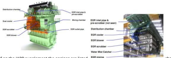
If on the IAPP supplement the engines are listed \_\_EGR mixing \_\_\_\_\_\_\_ should be determined, as it is important for clients to know if Selective Catalytic Reduction (SCR) or Exhaust Gas Recirculation (EGR) is in use.
