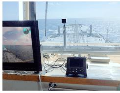
Head-Up-Display (HUD) / Augmented Reality (AG) units should be easily identifiable on the bridge and should be listed on the bridge equipment list.
